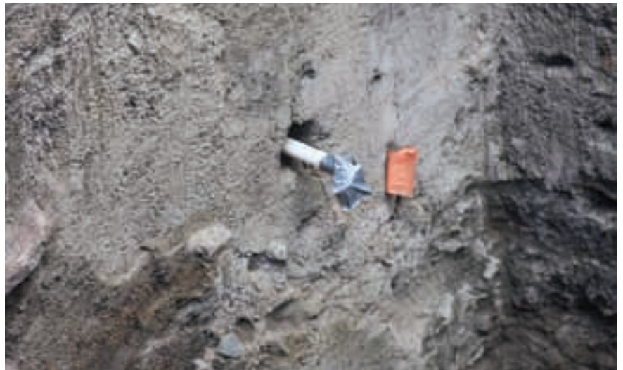
A tube-like measuring device, known as a dosimeter, is inserted into the wall of an excavation unit. It will take approximately a year for the dosimeter to take a luminescence reading of these deposits.
